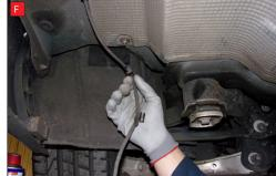
A) After you have removed O.E exhaust you will need to swap the valve motors to the Scorpion exhaust. Remove the 6 nuts
